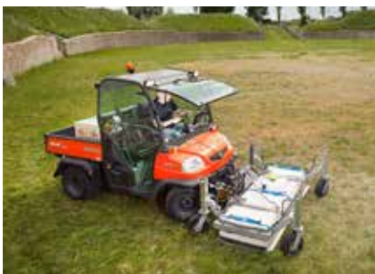
Figure 2 A motorised GPR array going over the ground above an amphitheatre
