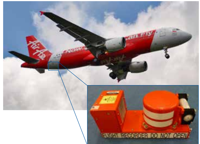
Figure 1 A black box flight recorder is normally located near an aircraft's tail, as this area generally suffers the least damage in an accident.
